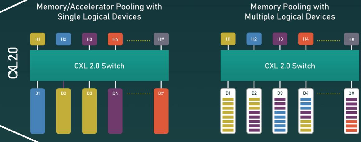
CXL 2.0 across Multiple Nodes inside a Rack/ Chassis supporting pooling of resources
