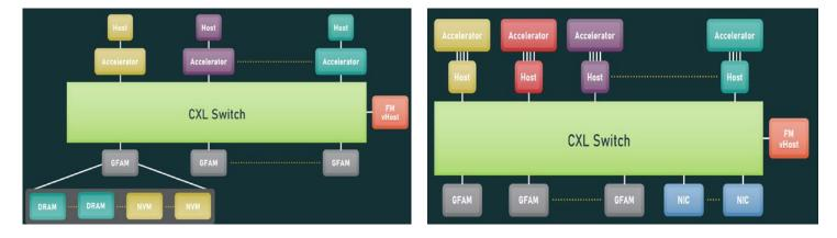
Figure 6: ML Accelerator & GFAM Device (left), HPC Analytics with Shared Memory and NIC (right)
