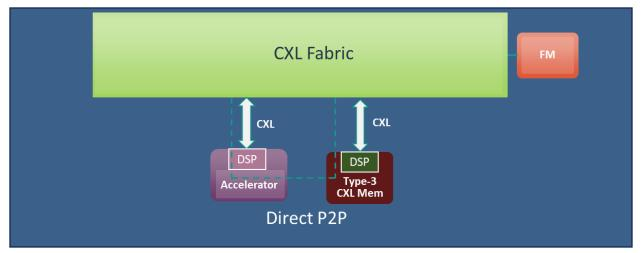
Figure 3: Direct P2P access of Accelerator to Type-3 Memory connected directly across a PBR switch
