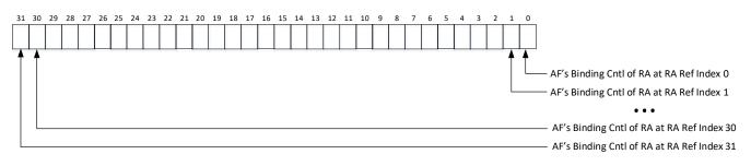
Figure 6-76: AF to RA Binding Control Entry
