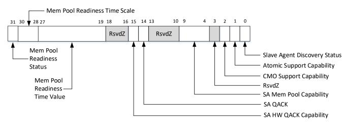
Figure 6-65: SACapStat Register at Byte Offset-04h
