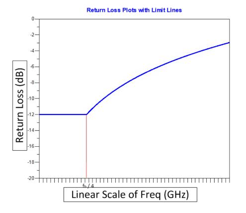
Figure 5-17: Channel Differential Return Loss Mask for EDR25-SR Link
