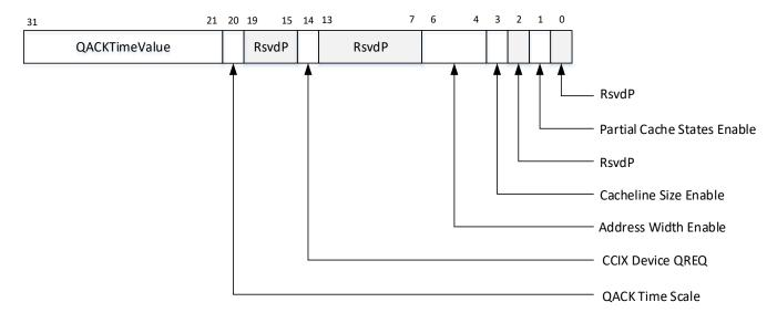
Figure 6-20: ComnCntl2 Register at Byte Offset-08h
