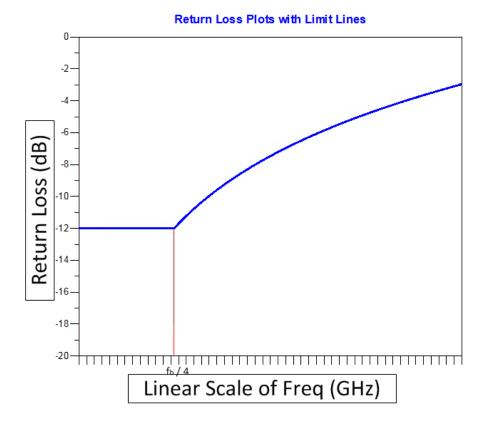
Figure 5-36: Channel Differential Return Loss Mask for EDR25-LR Link
