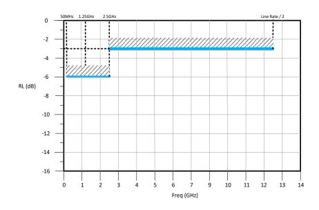
Note: The termination of the measurement is 250hm
