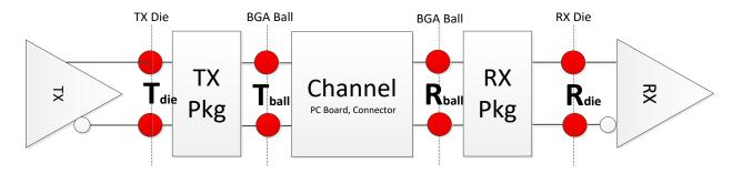
Figure 5-20: Reference Model of EDR25-LR Link
