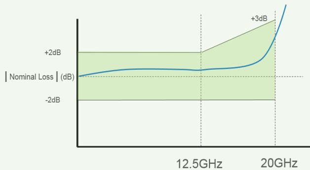
Figure 5-9: The frequency mask of combiner block
