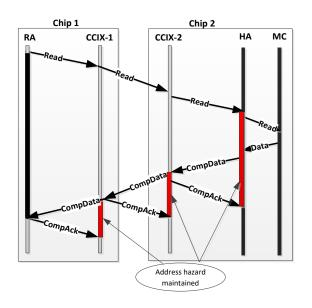
Figure 3-35: Example of a Read Transaction Flow
