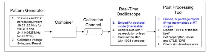
Figure 5-12: General Flow for Using Post Processing Tool
