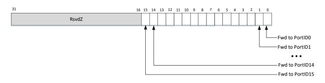
Figure 6-35: PortCapStat3 Register at Byte Offset-0Ch
