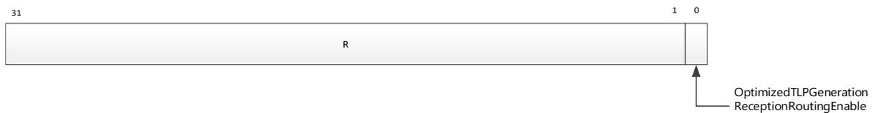
Figure 6-85: TransactionLayerControl Register
