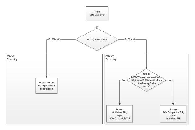
Figure 4-6: CCIX Transaction Layer Received TLP Processing Flow
