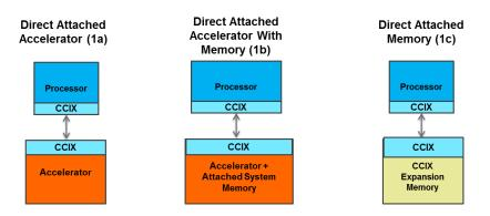
Figure 2-1: Example CCIX Direct-Attached topologies
