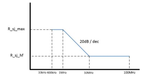
Figure 5-26: Jitter Tolerance Mask of EDR25-LR PHY
