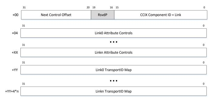
Figure 6-44: CCIX Link Control structure
