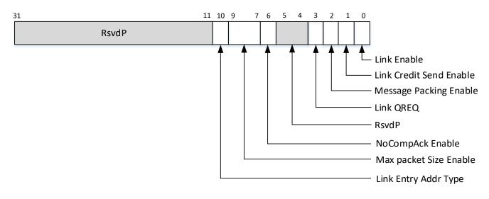
Figure 6-46 shows the layout of the CCIX Link Attribute Control (LinkAttrCntl) Entry at Byte Offset-00h.
