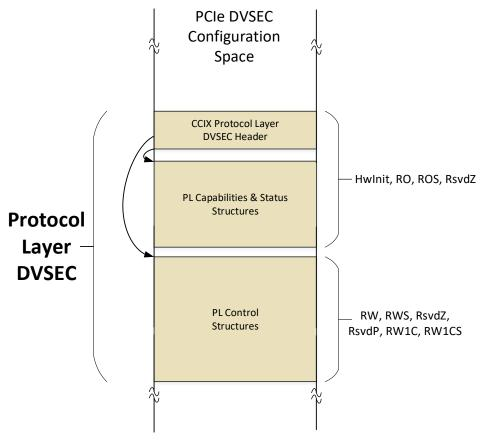
Figure 6-3: CCIX Protocol Layer DVSEC structure types
