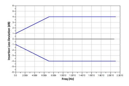
Figure 5-37: Insertion Deviation Mask for EDR25-LR PHY
