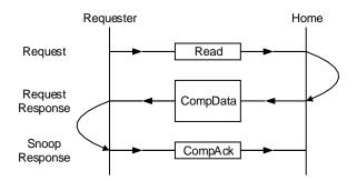
Figure 3-4: Coherent Read transactions with CompAck
