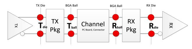
Figure 5-1: Reference Model of EDR25-SR Link
