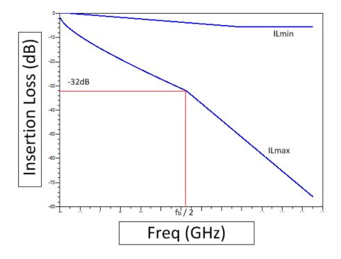
Figure 5-35: Insertion Loss Mask for EDR25-LR
