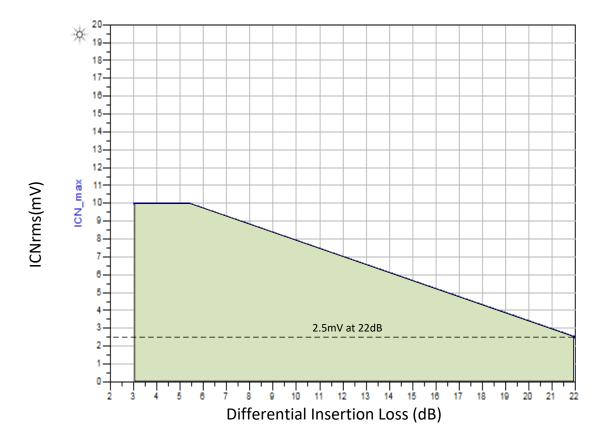
Figure 5-19: ICN<sub>rms</sub> Mask vs Insertion Loss
