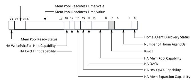
Figure 6-54: HACapStat Register at Byte Offset-04h
