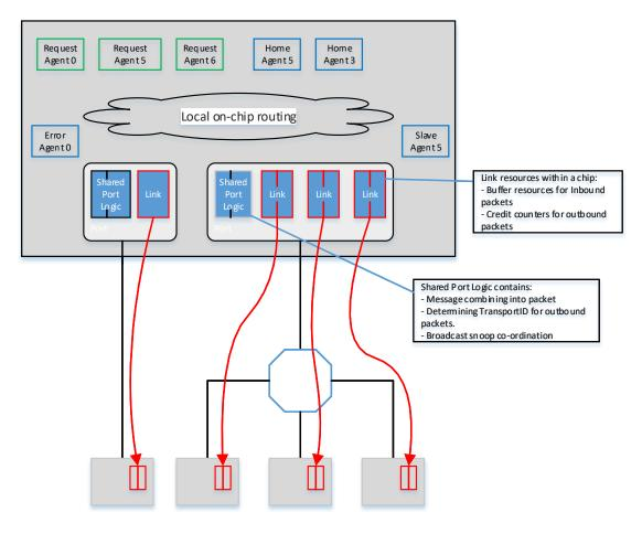
Figure 3-1: Illustrating CCIX Components
