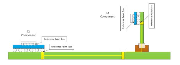
Figure 5-2: Reference Points on a downstream direction of EDR25-SR link
