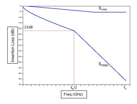
Figure 5-16: Insertion Loss Mask for EDR25-SR Link
