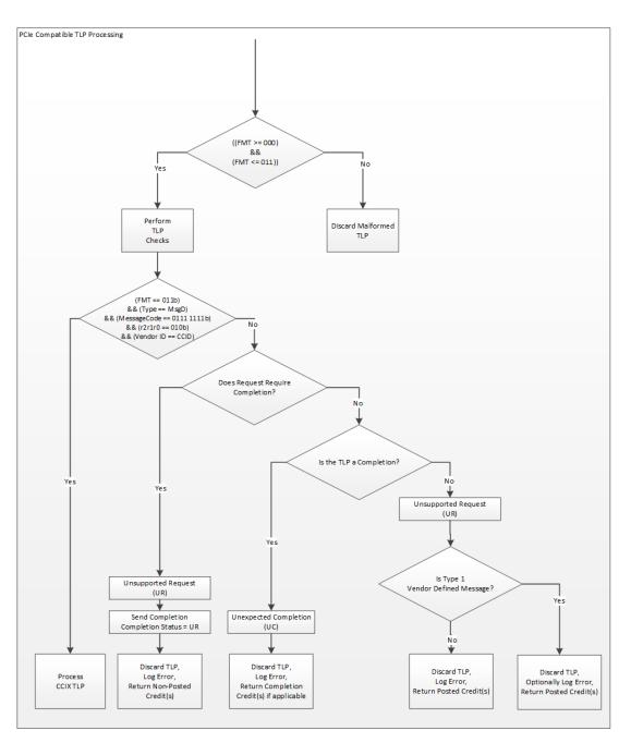
Figure 4-7: PCIe Compatible TLP Processing Flow
