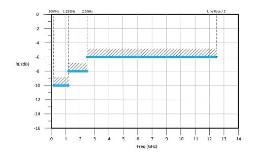
Note: The termination of the measurement is 100ohm
