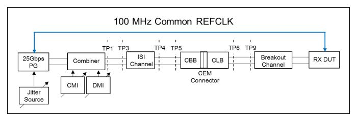
Figure 5-13: Layout for Jitter Testing for Common Refclk Rx
