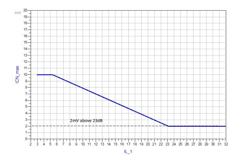
Figure 5-38: ICN<sub>rms</sub> mask vs Insertion Loss
