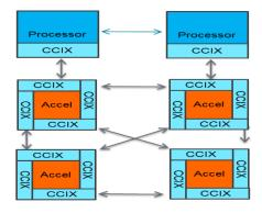
Figure 2-2: Example CCIX Fully Connected topologies
