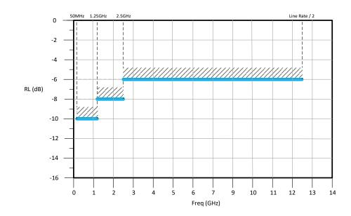
10 The receiver differential return loss at R<sub>ball</sub> including package and socket is given in the Figure 5-3.
