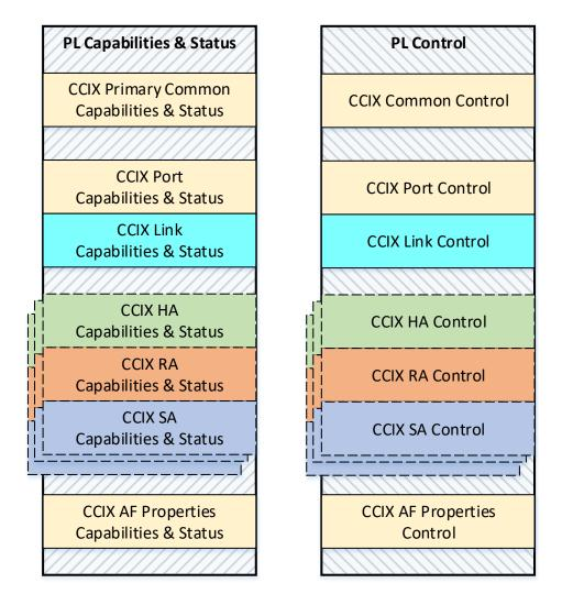
Figure 6-7: Sequence of CCIX Protocol Layer Component Structures
