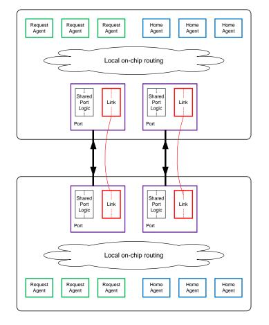
Figure 3-32: A two Chip Topology with Example Internal CCIX Components
