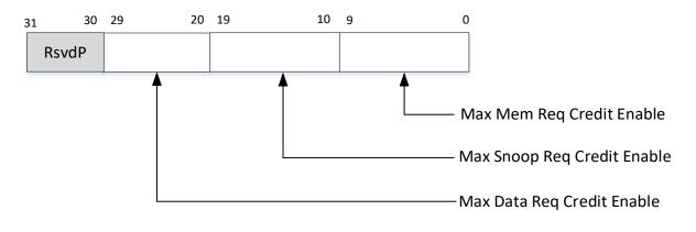
Figure 6-47: LinkMaxCreditCntl Entry at Byte Offset-04h
