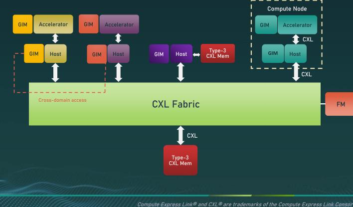
Host to Fabric-Attached Memory (FAM) communication with Global Integrated Memory (GIM)
