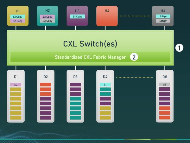
1 Expanded use case showing memory sharing and pooling
