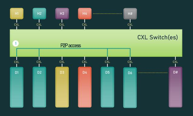
1 CXL 3.0 enables efficient peer-to-peer communication (P2P) between devices. Relies on PCIe Unordered I/O.
