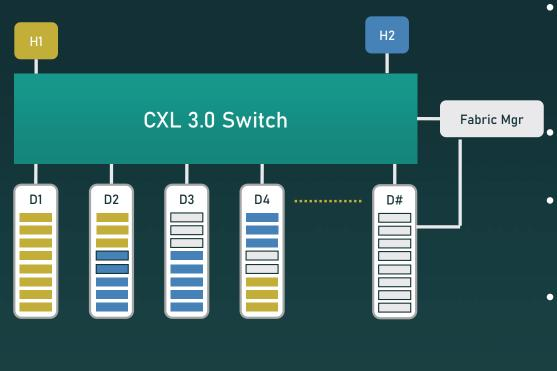
Memory Pooling allows a host to dynamically expand/shrink its memory capacity to match Workload
