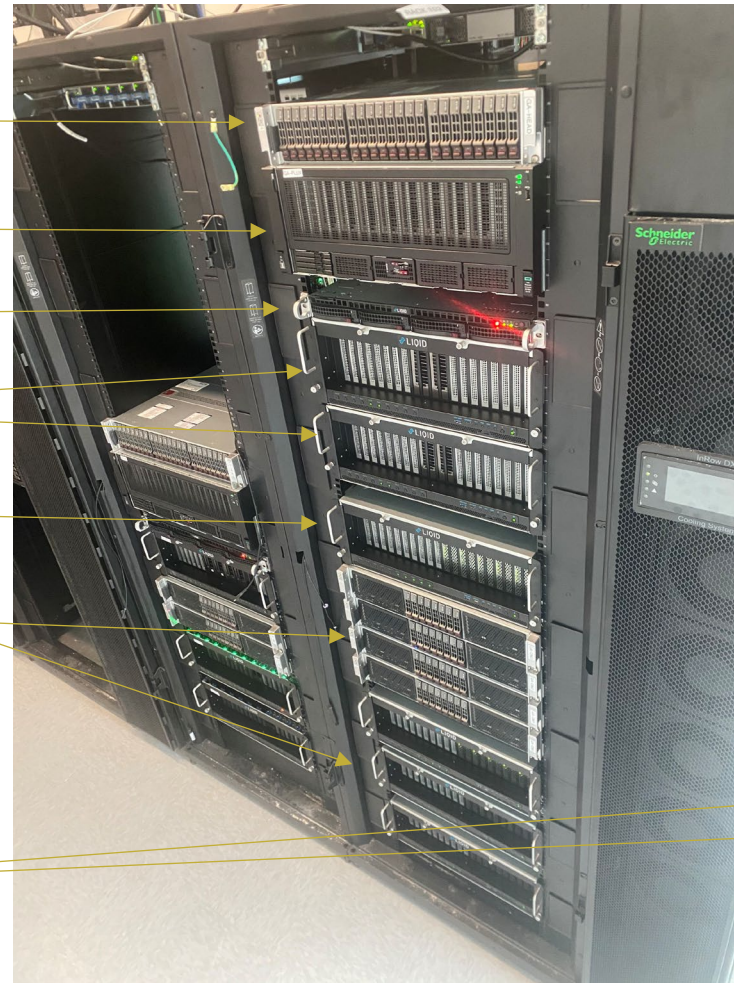
Front of Rack (Cold side)
